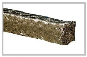
RassTech RCP 110 G-1 is braided from pure expanded mineral graphite twisted yarn with exceptionally low carbon content. This results in long-lasting packing, featuring a low coefficient of friction, excellent heat transfer properties and exceptional chemical resistance.
